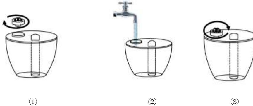
3. Screw down the lid and put the water tank back on to unit properly.
